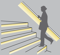
Handrail light, foot lights for stairs
