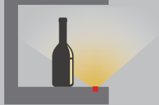
Illuminate the object from the bottom of the showcase.
